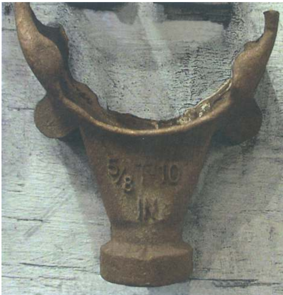
Fig. 5-9. A red brass casting shows a short pour and inadequate volume.
