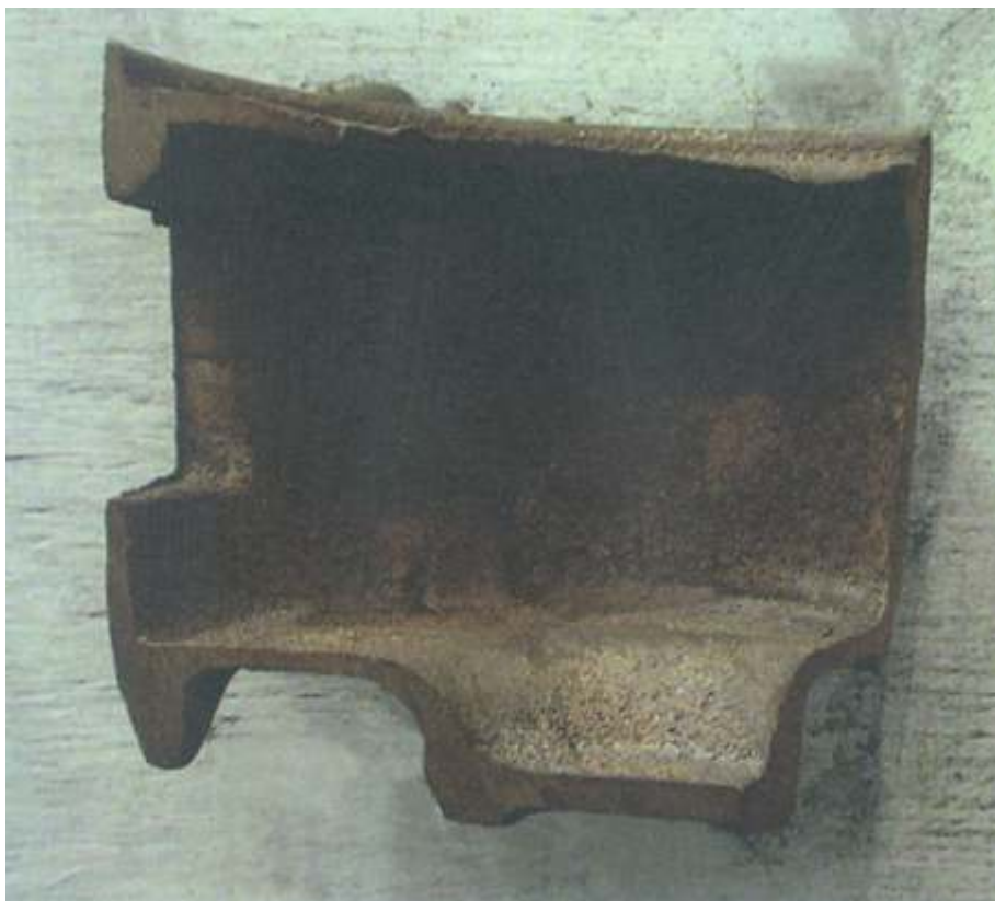
Fig. 4-18. Core lift results from inadequate placement; worn core prints allow 'float' in the mold.
