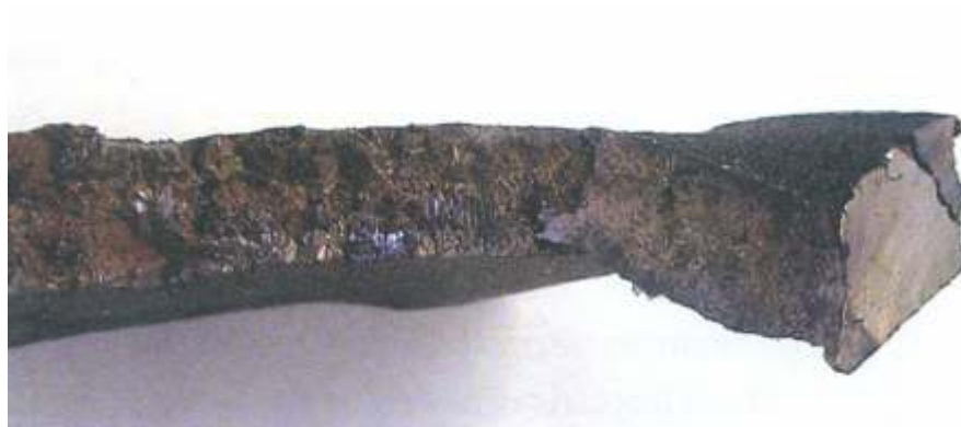
Fig. 6-8. Hot tear in a leaded semi-red brass.
