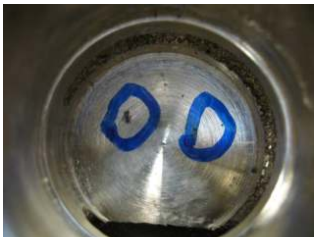
Fig. 12-5. Defect areas at the bottom of the large bore.
