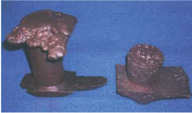
Fig. 7-16. The 'mushrooming' copper casting is due to high gas content in the melt.
