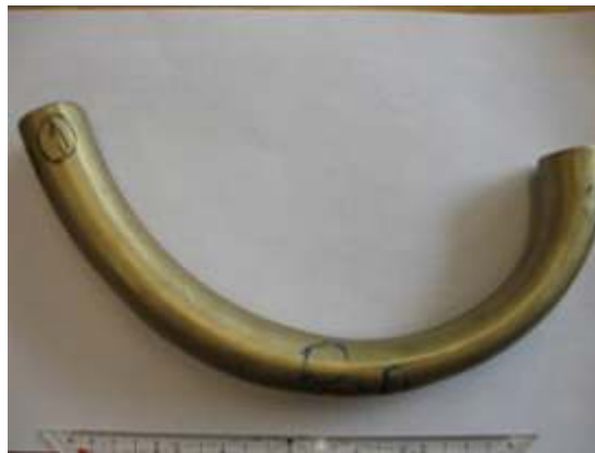
Fig. 12-1. Object 1, exhibiting surface cracks and a surface bulge at the location indicated by the circle at the right border of the image.
