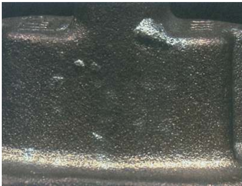
Fig. 11-3. Red brass exhibits tin sweat, caused by long solidification and gas evolution. Proper degassing and directional solidification are remedies.
