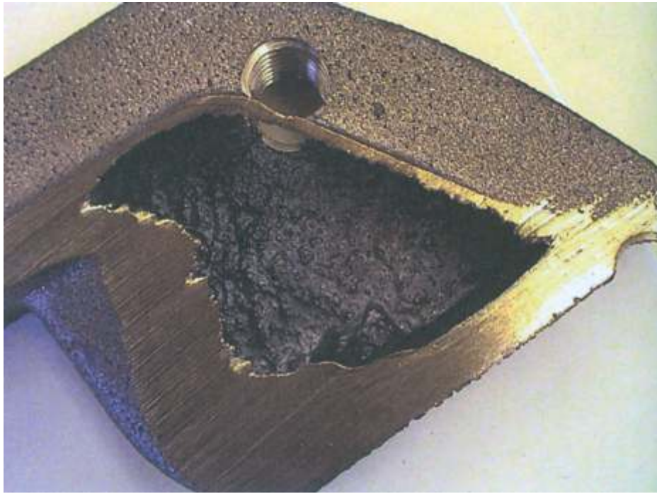
Fig. 7-14. A gross blow and dispersed porosity in red brass is the result of a wet core adhesive and improper venting.
