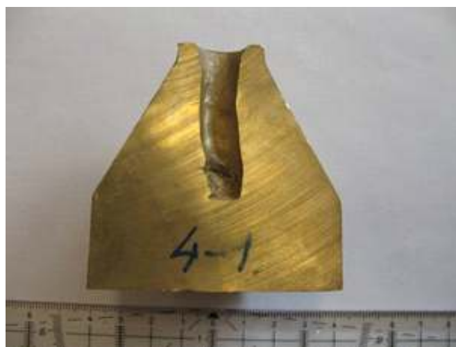
Fig.12-8. Object 3, a cone-shape casting with a blind hole at the center.
