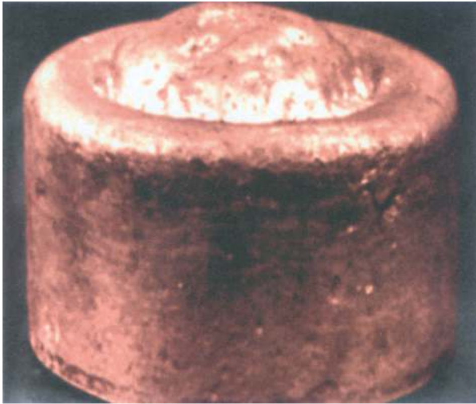
Fig. 7-1. A rise is associated with gas porosity in the casting.
