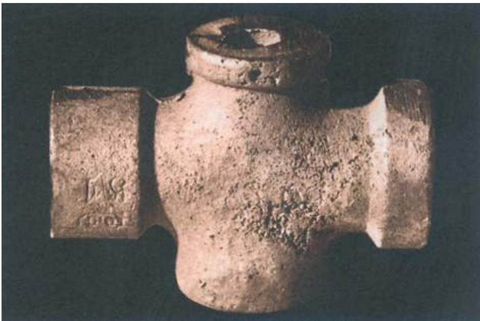
Fig. 10-2. Bronze valve body cast in green sand shows sand inclusions caused by core erosion.
