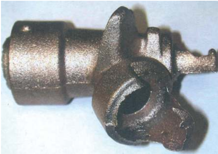
Fig. 4-16. Improper core alignment in red brass.
