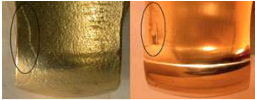
Fig. 13-4. A graphite wake type surface defect before and after grinding.
