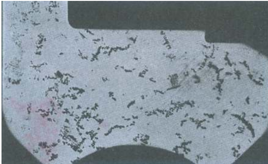
Fig. 7-3. A bronze casting displays macro-porosity.
