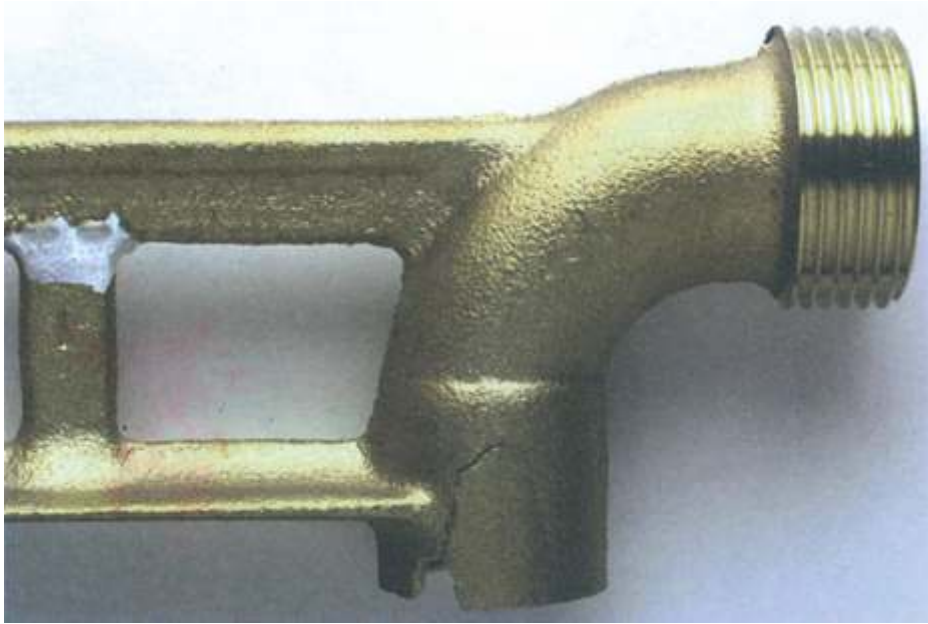
Fig. 11-4. Yellow brass casting crack, observed after machining, is possibly due to severe residual stress and/or temperature state during machining.
