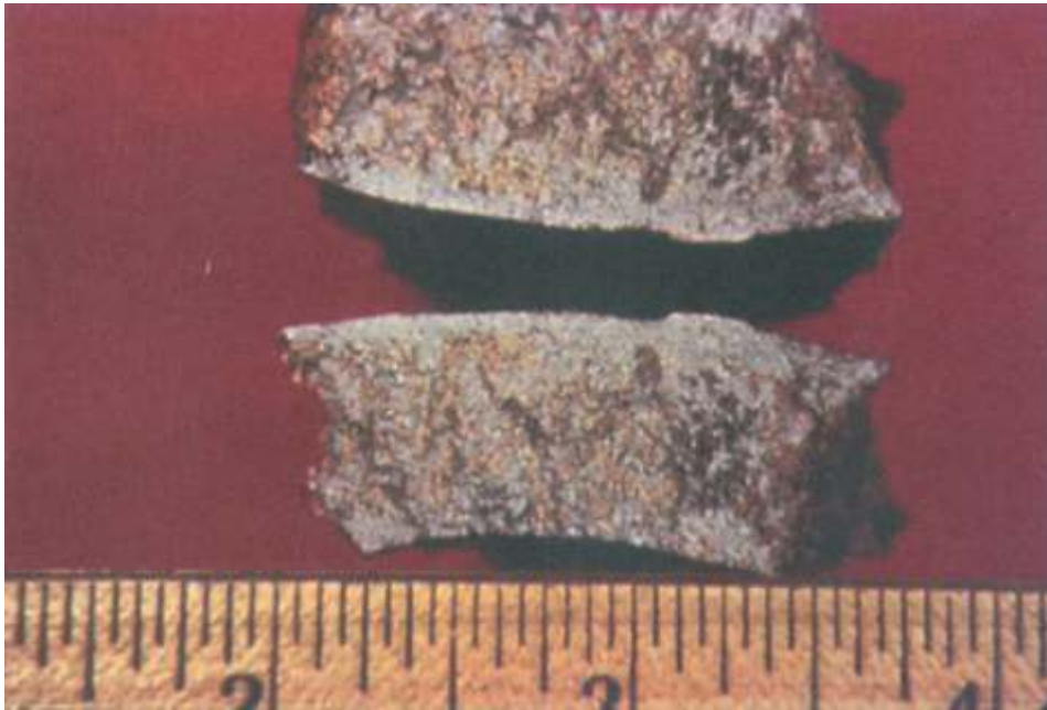
Fig. 1-2. Silicon in red brass is an impurity concentration that results in casting microstructural weakness prone to cracking.
