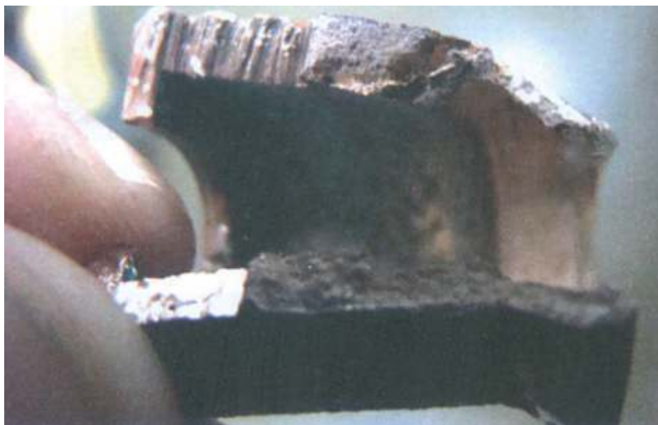
Fig. 8-4. Severe macro shrinkage in leaded red brass is caused by too low of a pouring temperature and/or insufficient feeding.
