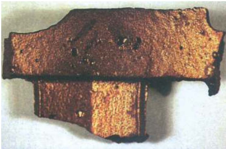
Fig. 7-17. Heavy section brass casting exhibits gas blow during final solidification. Potential solutions are de-gas; provide better feeding; use of chills and lower pouring temperature.
