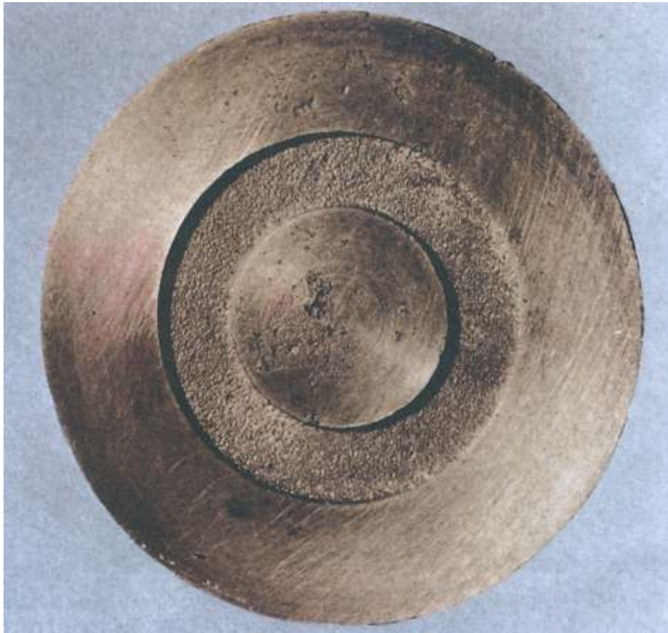
Fig. 10-1. Brass casting contains dross inclusions.
