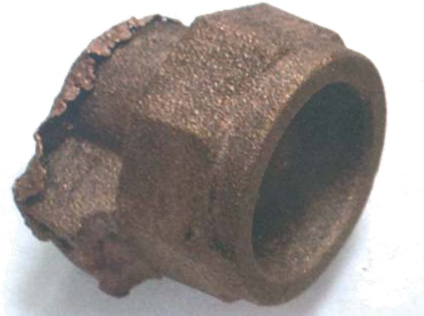
Fig. 4-5. Swell is caused by cracked sand mold in red brass (C83600).
