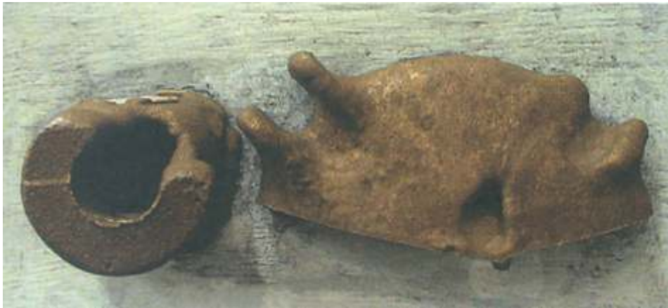
Fig. 5-8. A misrun in red brass is caused by low temperature, inadequate gating and low phosphorus deoxidation.
