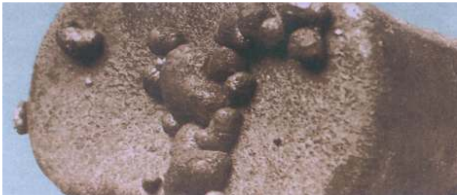
Fig. 11-1. Leaded tin bronze cast in green sand. Sprue exhibits tin sweat.
