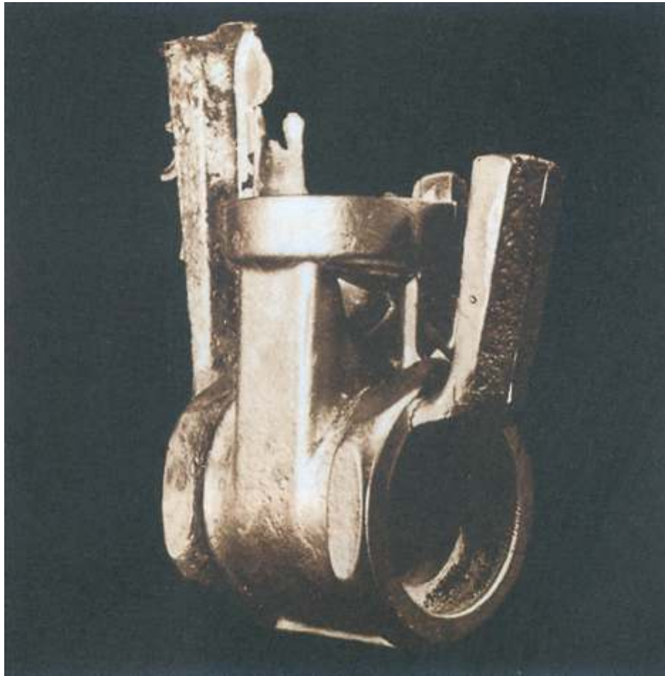
Fig. 5-3. A brass valve body cast in permanent mold shows a misrun caused by entrapped air.
