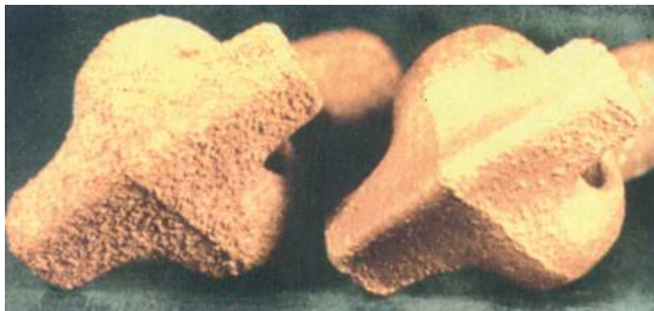
Fig. 9-4. The casting shows a burn in or metal penetration caused by improper sand mixture, excessive metal fluidity, and pouring temperature.
