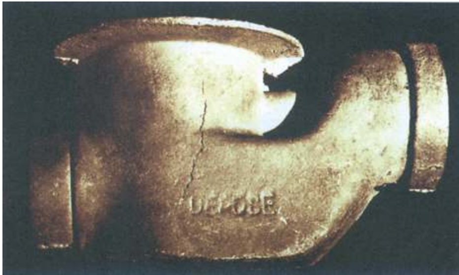
Fig. 6-3. The hot tear in the brass valve body in green sand is due to restrained contraction and excessive pouring temperature.
