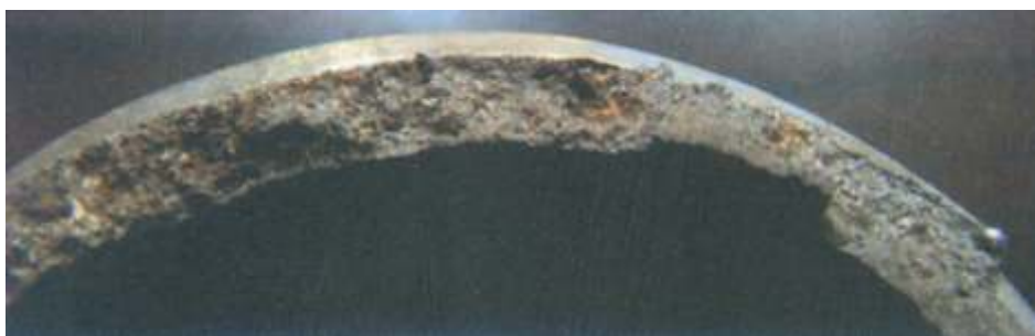
Fig. 8-5. Shrinkage porosity in red brass is caused by poor solidification (low pouring temperature, inadequate feeding).
