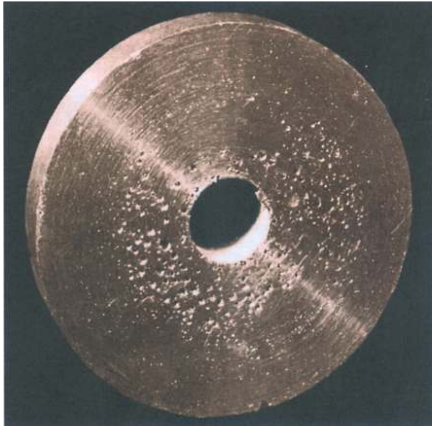
Fig. 7-4. Tin bronze alloy cast in dry sand has blowholes due to gassy melt.
