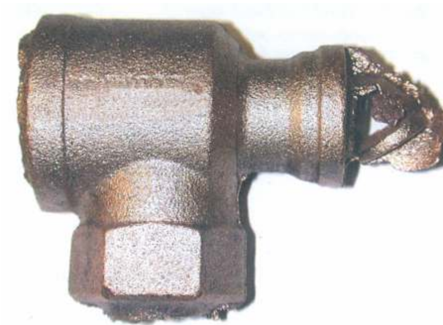
Fig. 4-17. Improper core placement in red brass.
