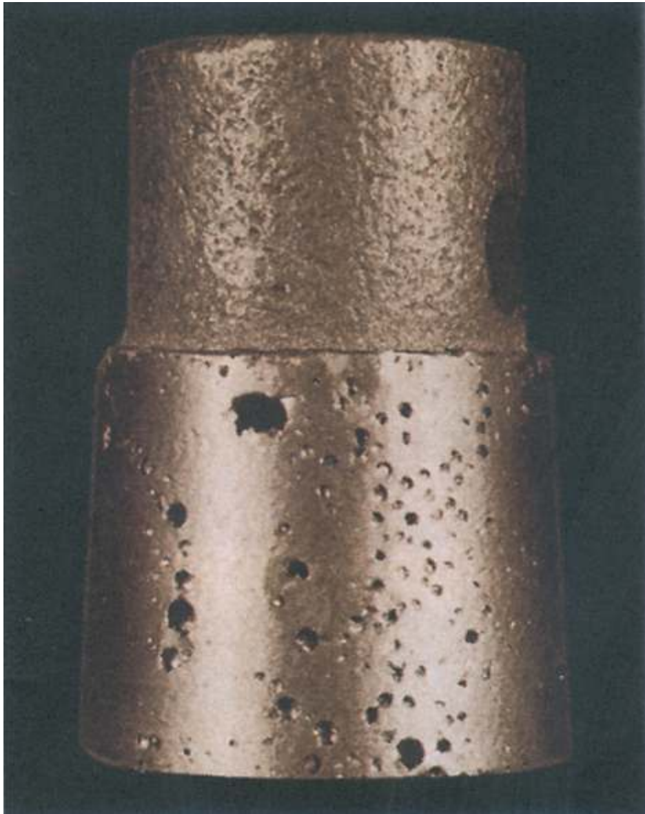
Fig. 7-5. Bronze stopper cast in green sand has blowholes due to gassy melt and/or mold/metal reaction with excessive moisture in the sand.
