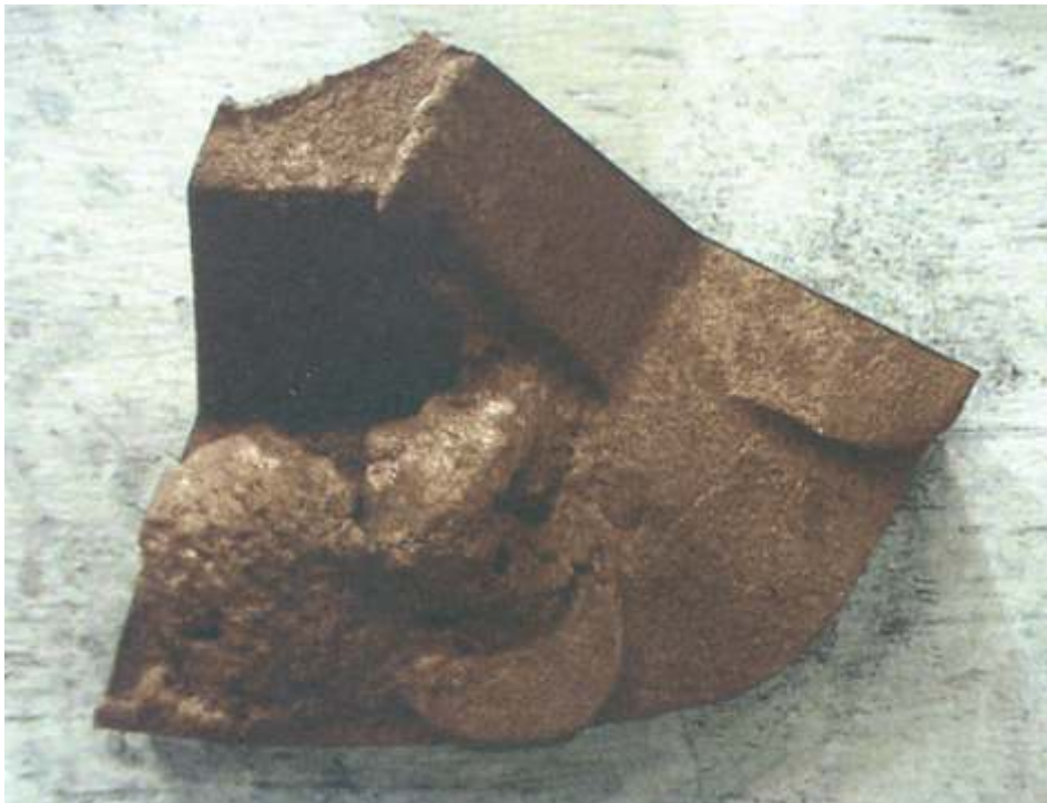
Fig. 1-5. The cracked mold is caused by push up or drop. The drag sand level is not full.
