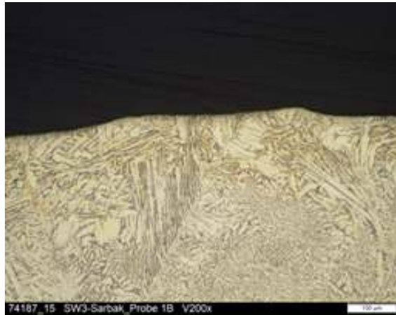
Fig.12-13. Target cross section through the surface bulge at Object 1.
