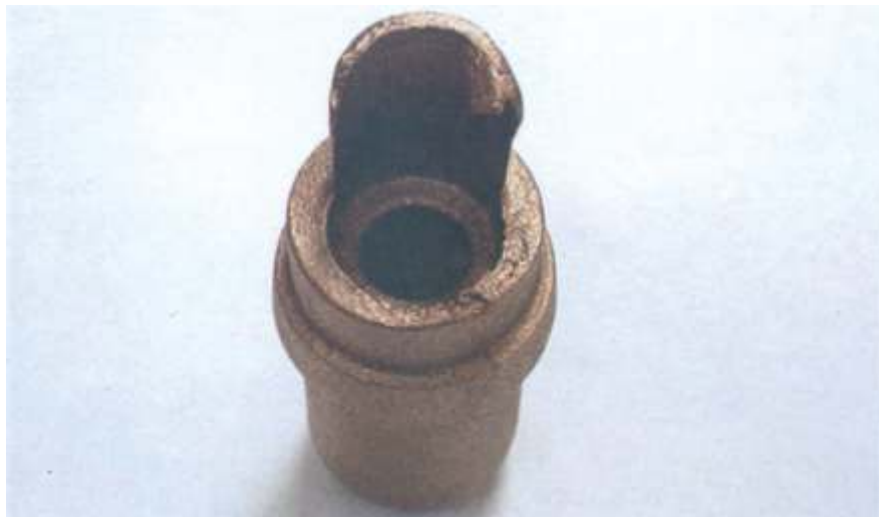
Fig. 4-15. Dimensionally incorrect core in red brass results in crush.
