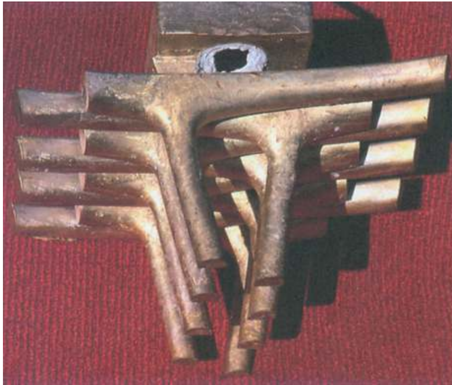
Fig. 10-7. Poor surface on aluminum bronze casting is due to excessive dross formation and lack of removal prior to pouring.
