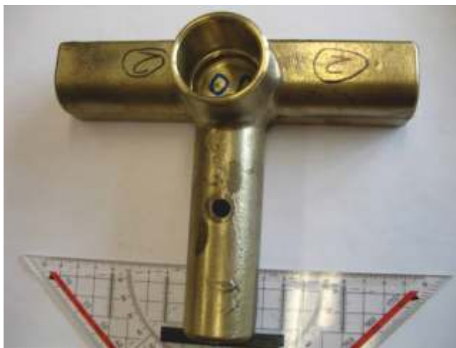
Fig. 12-4. Object 2 (body of a drain valve). At the bottom of the large bore in the center of the cast body, two defect areas were detected.
