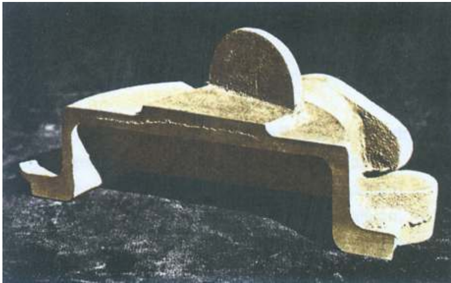
Fig. 8-1. Brass sand casting shows centerline shrinkage crack. Lowering iron and tin content, increasing riser size and reducing pouring temperature would eliminate the shrink.
