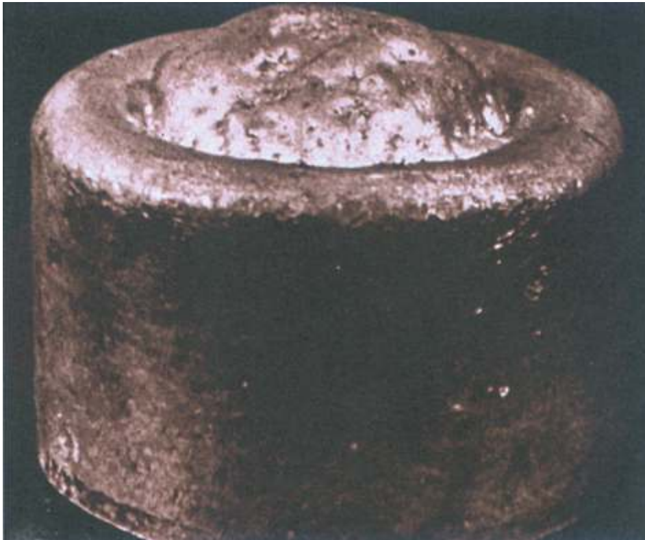
Fig. 7-12. A copper base casting shows a 'mushroom' gas evolution.
