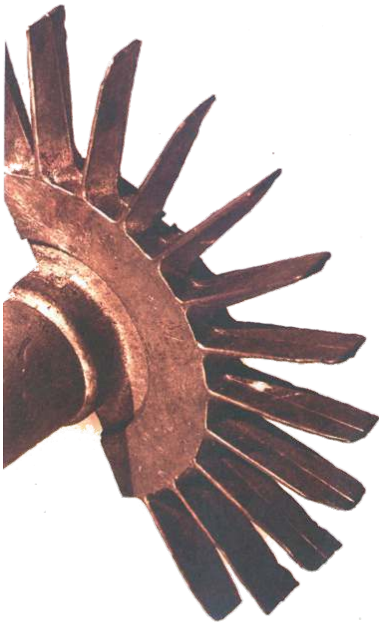
Fig. 5-2. A cupro-aluminum permanent mold casting exhibits a misrun due to lack of venting.
