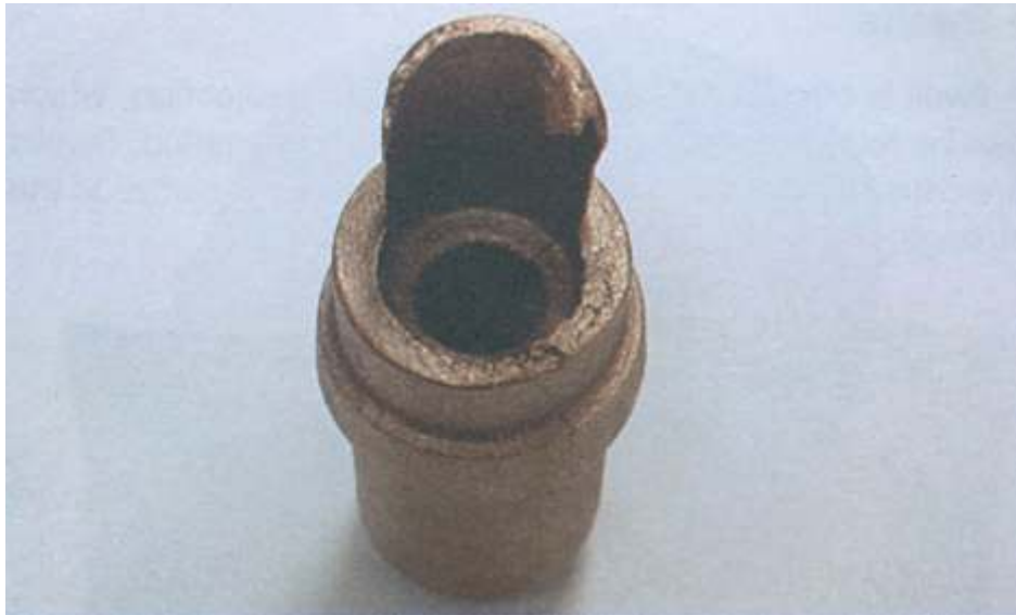
Fig. 4-2. Core crush from insufficient core strength.
