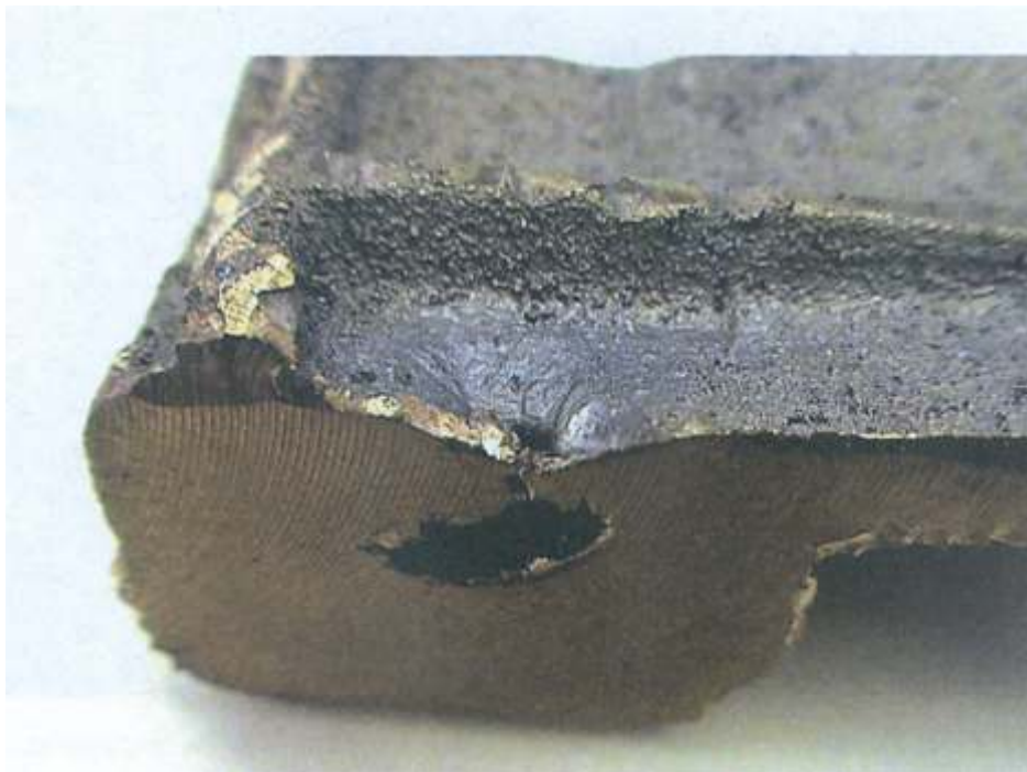
Fig. 7-13. A core gas blow in leaded red brass is the result of poor venting and pouring temperature being too high. Also, inadequate gating causes localized heating at a thick section and a concentrated gas blow within the casting.
