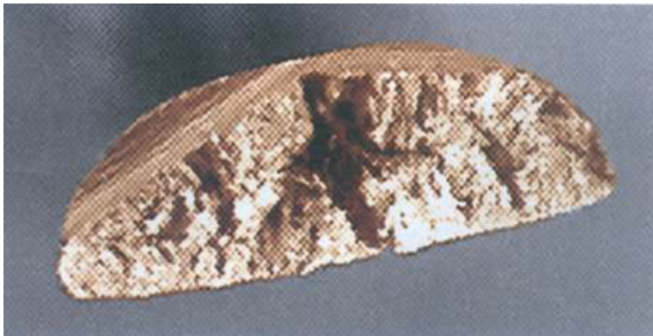
Fig. 6-4. A fracture in red brass cast in green sand exhibits excessive dendrite growth due to excessive melt and/or pouring temperature; venting helps.
