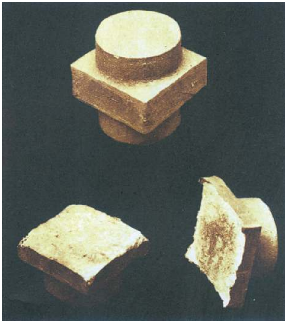
Fig. 5-1. A bronze screw nut cast in green sand shows effect of interrupted pouring.
