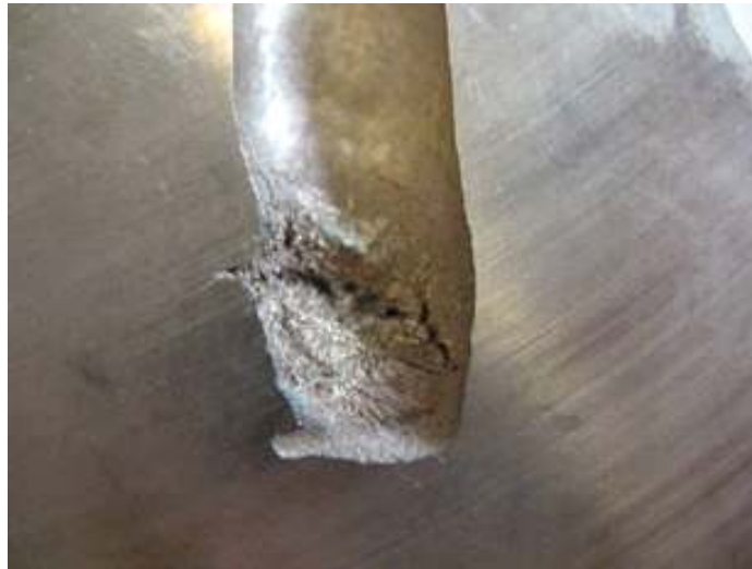
Fig.12-9. Defect area inside the blind hole.
