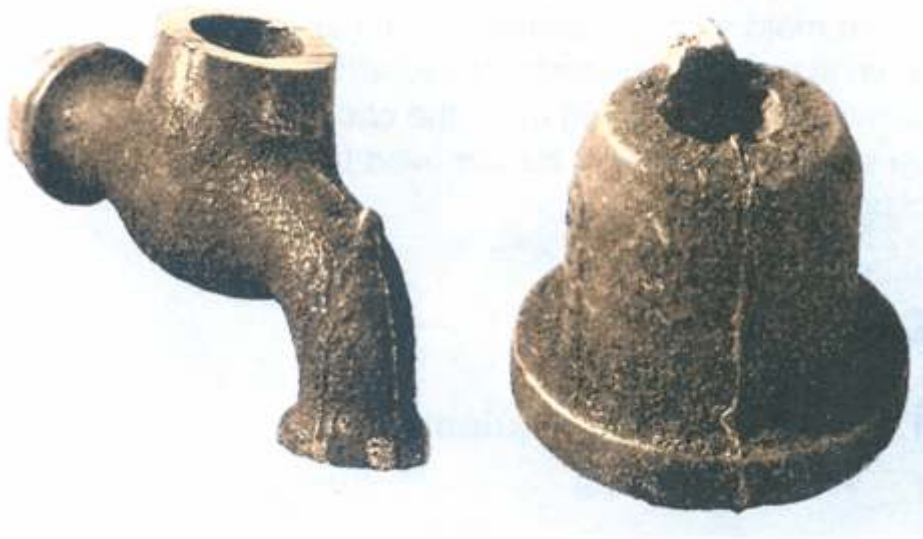
Fig. 9-1. A bronze alloy in green sand exhibits burn-on.
