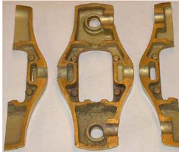
Fig. 13-2. Example of the cutting of the last casting in each sequence.
