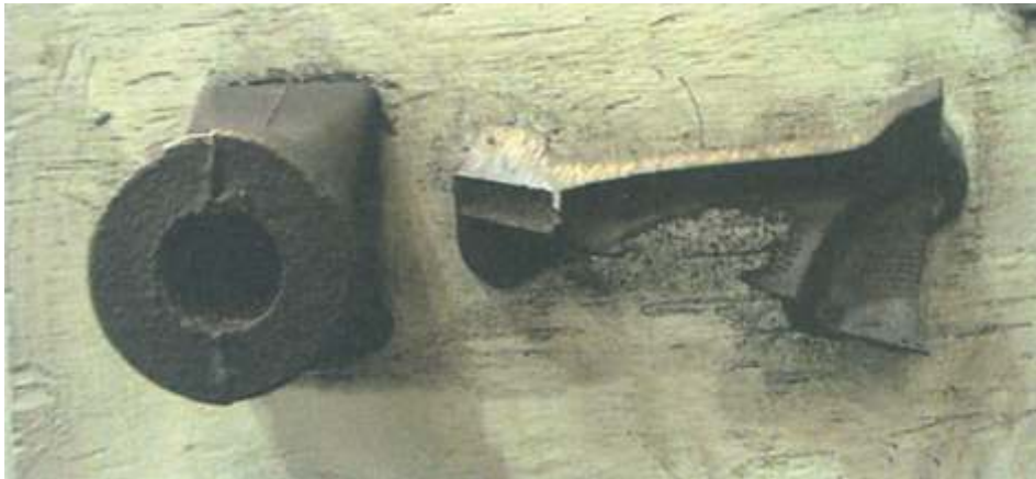
Fig. 1-4. The broken core shows low binder content, poor density and age.
