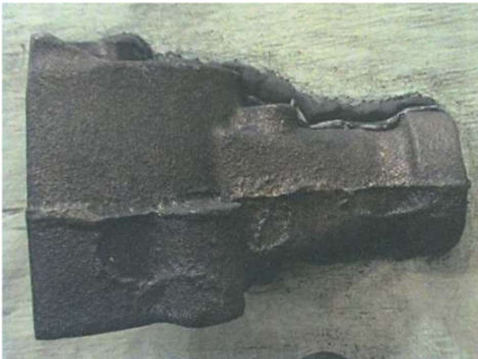
Fig. 4-3. Crush can be caused by misaligned cope/drag, mismatched pattern halves, bad pins, and bushings.
