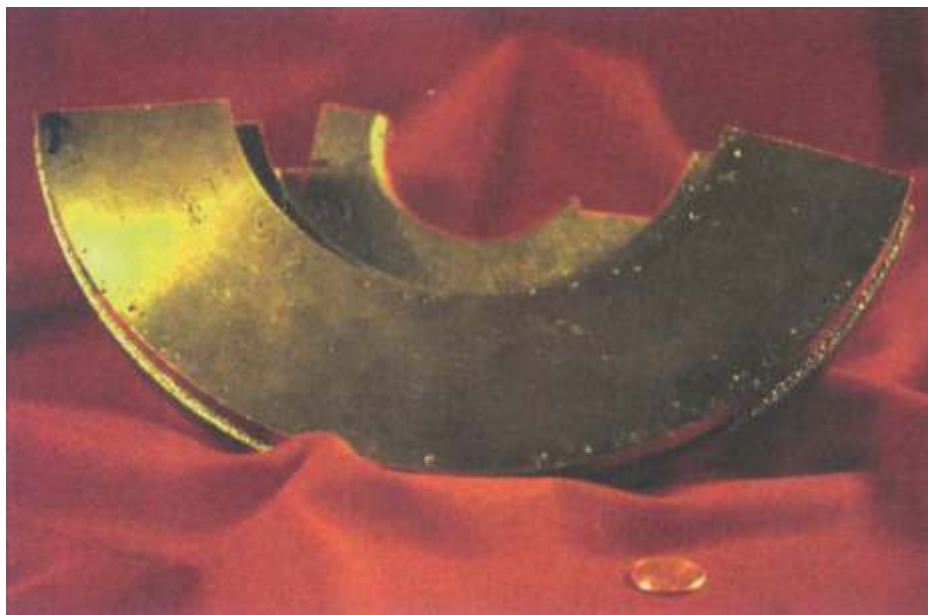
Fig. 7-15. Pinholes in aluminum bronze result from inadequate degassing.
