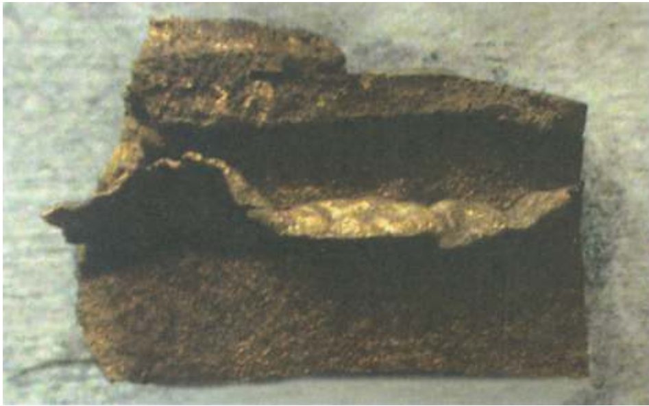
Fig. 3-13. Severe veining in red brass C83600.
