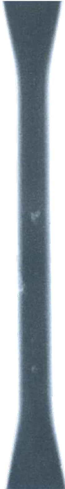
Fig. 7-10. X-ray of cast test bar exhibits gross porosity in brass.
