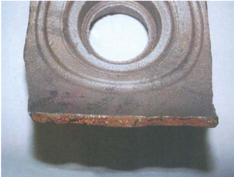
Fig. 6-5. Hot tear in red brass caused by shakeout, which is too soon and/or too hot.
