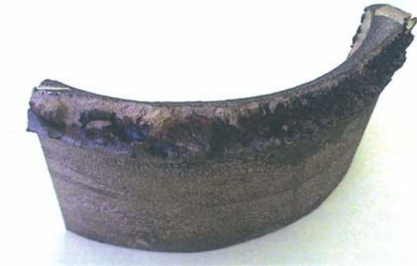
Fig. 6-7. The hot tear in red brass resulted from the binder content being too high and from mold restraint.
