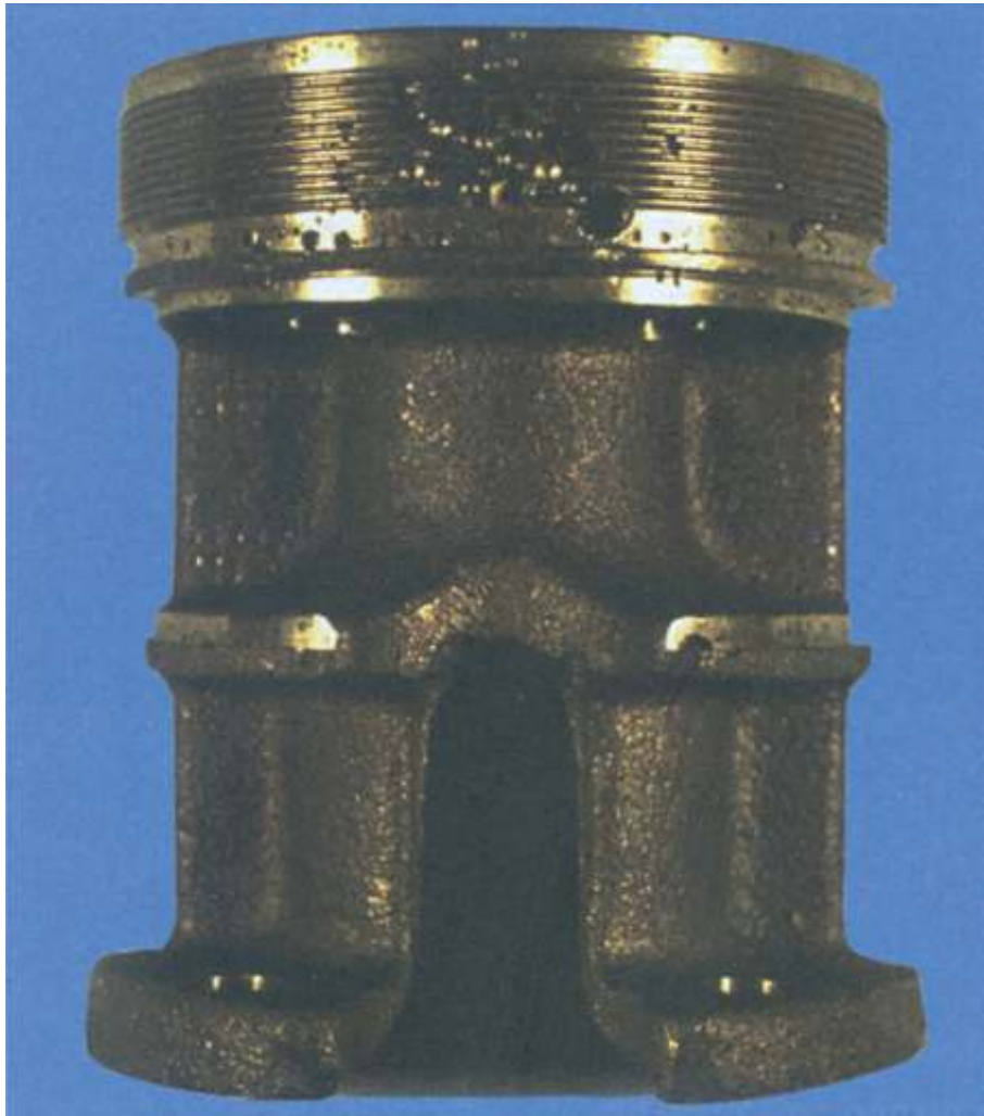
Fig. 7-11. Severe gas porosity is seen in red brass.
